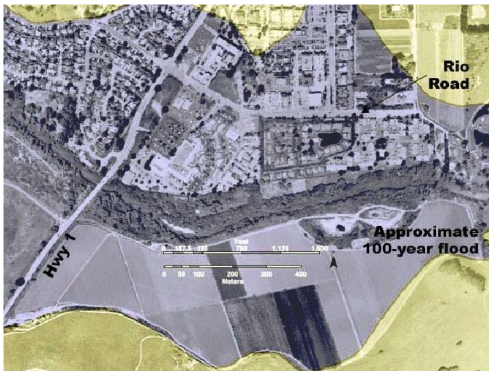
Figure 2-15C. Example of urban development in the lower Carmel River that would be affected by the estimated 100-year flood. Approximate affected area shown in blue (FEMA 1996). Levees exist along both sides of the Carmel River upstream (right) of Highway One. Background photo from MEI (2002) (Smith 2004).
